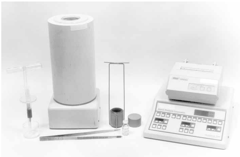
Figure 6.3. A photograph of a radionuclide calibrator with its signal processing equipment and printer. The plastic inset serves to position vials or other radioactive sources where required.
